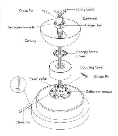
WARNING: The tab in the ring must rest in the groove of the hanger ball/downrod assembly. Failure to properly seat the tab in the groove could cause damage to the wiring.
